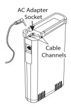
Note: WeatherLink Live is powered by AC power with battery backup. **AC power is required; it cannot be set up or run on batteries alone.** It is highly recommended that you install batteries to prevent loss of data if AC power is lost.
