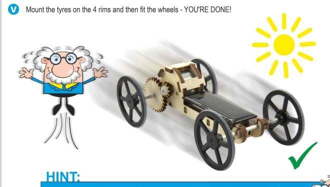
The Solar-Runner is best to drive in **direct sunlight**. We therefore recommend that you test the Solar-Runner outside in good weather. If the Solar-Runner is not able to get into gear despite sunlight, check that the front and rear axles rotate freely. Now have fun and enjoy the ride!
