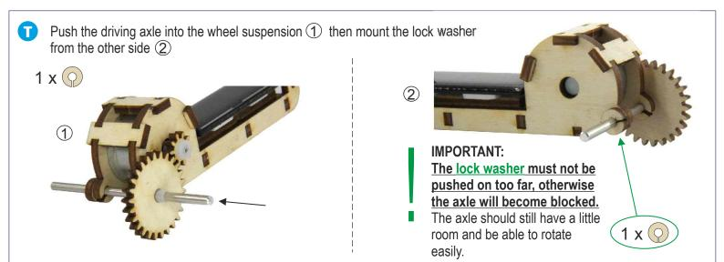
U Slide the remaining axle into the wheel suspension and fit it with 2 lock washers. The axle must still be able to rotate easily so do not push too far together.
